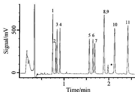
**Fig. 2** A chromatogram obtained from a 1 µl injection of a standard pesticide calibration mix at the 100 ng ml<sup>-1</sup> level. Split ratio was 10:1. Peaks: 1 = TCMS, 2 = α-BHC, 3 = β-BHC, 4 = δ-BHC, 5 = *cis*-chlordane, 6 = *trans*-chlordane, 7 = *p,p'*-DDE, 8 = *p,p'*-DDD, 9 = endrin, 10 = endosulfan sulfate, 11 = endrin ketone, \* = endrin aldehyde.
