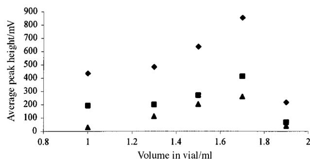
**Fig. 3** Plots to show how peak heights vary with volume of solution contained in the 2 ml vial.  $\diamond$ , *cis*-Chlordane;  $\blacksquare$ ,  $p,p'$ -DDD;  $\blacktriangle$ , endosulfan sulfate.
