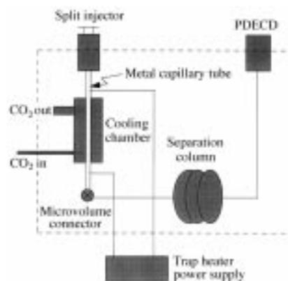
Fig. 1 Schematic representation of the experimental layout.
